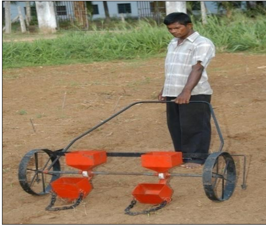
Manual Seeder for maize, green gram, black gram and soybean Photo Credit: FMRC
